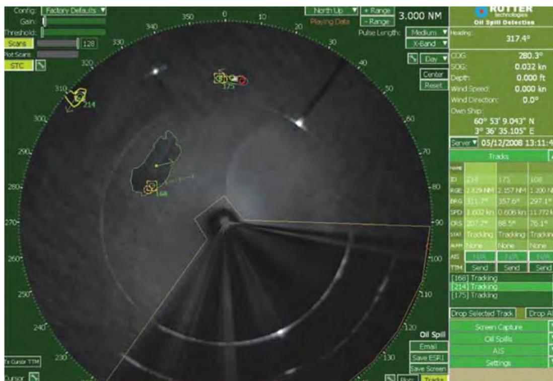
**Figure 5-6: Radar Signature of Oil on Water<sup>10</sup>**
