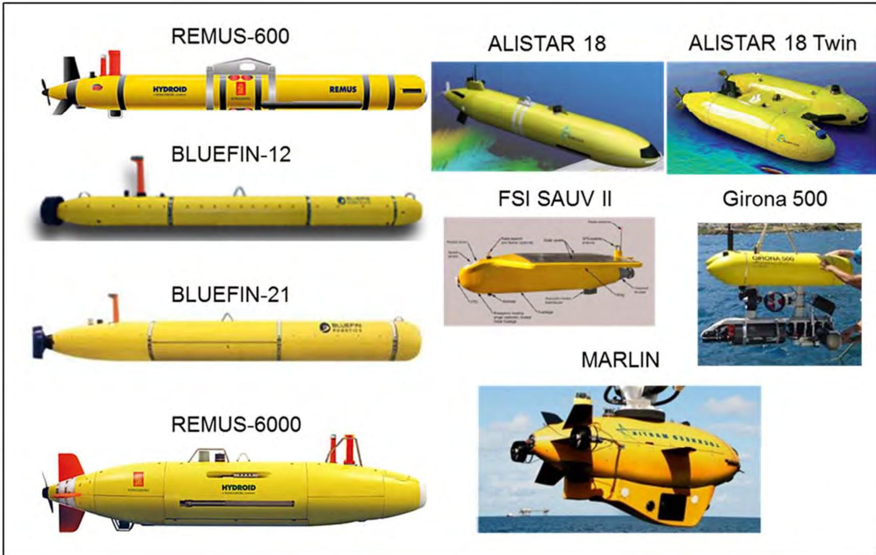
Figure 3-3: LWV and HWV Class AUVs
