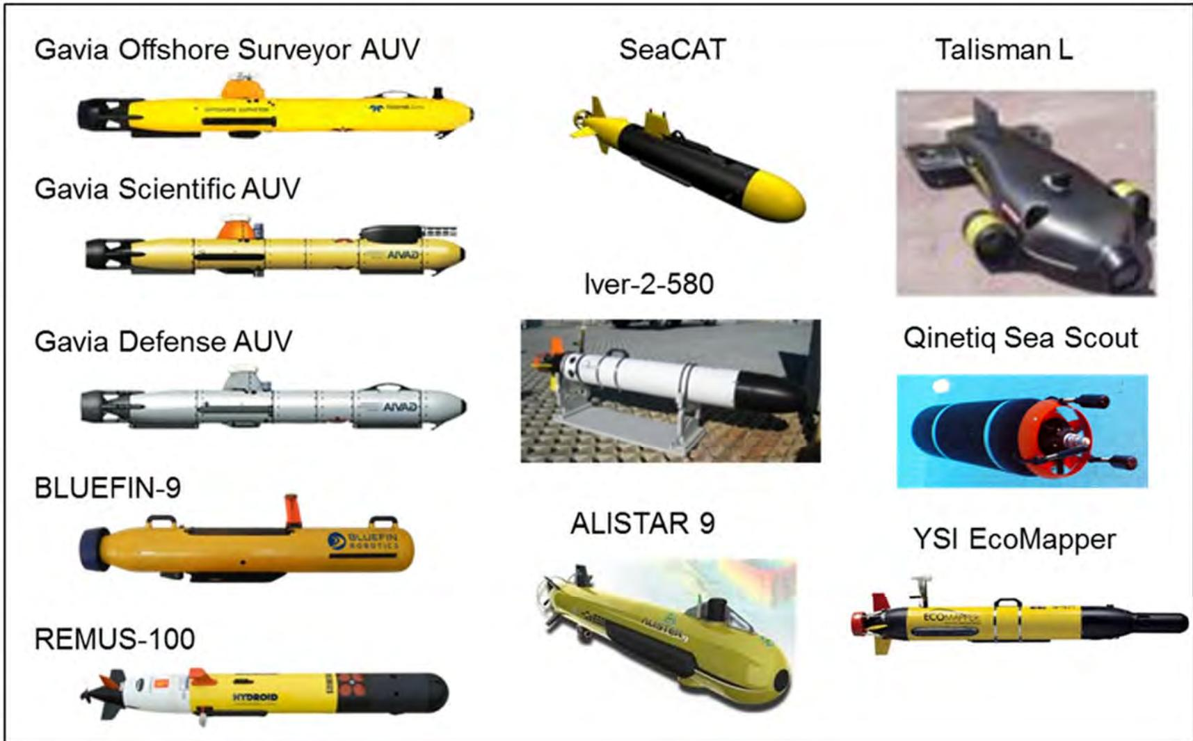
Figure 3-1: Man-Portable AUVs
