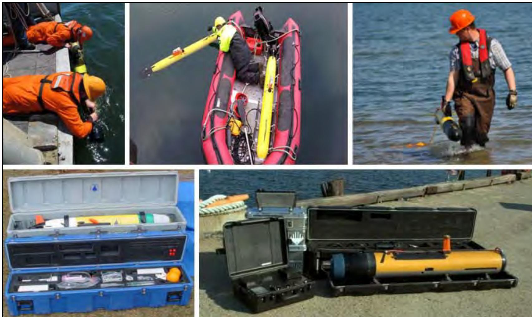
Figure 3-2: Man-Portable AUV Launch and Recovery and Stowage
