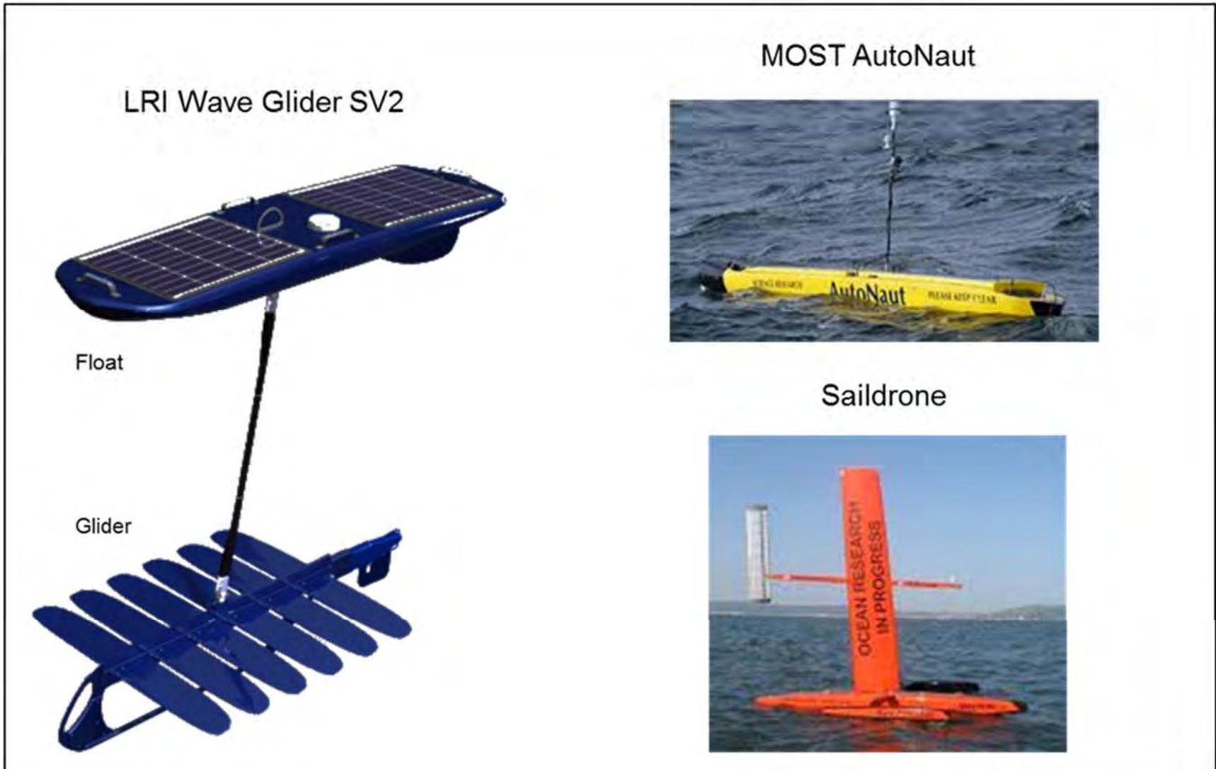
Figure 3-10: Wave and Wind Powered ASVs
