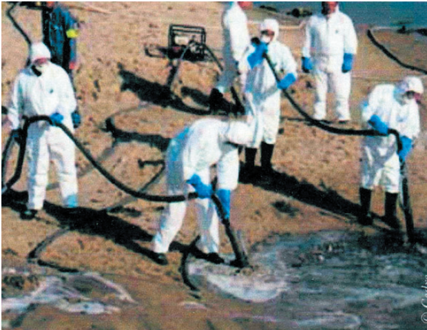
Flushing allows selective recovery of oil without taking too much sediment.
