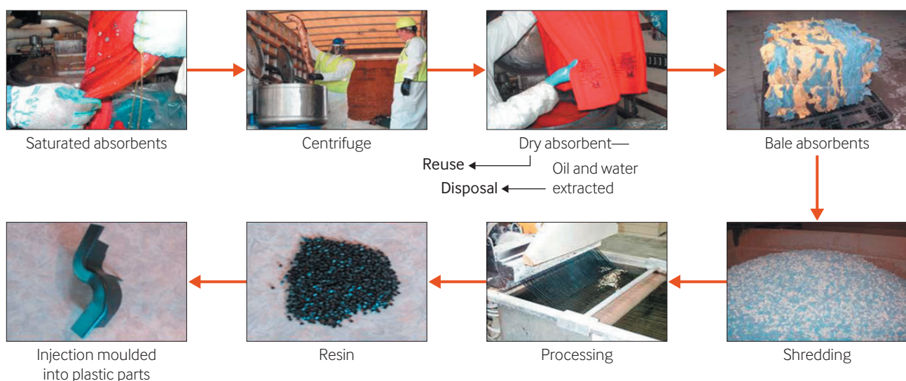
Figure 8: Illustration of a recycling process from boom material to plastic products
