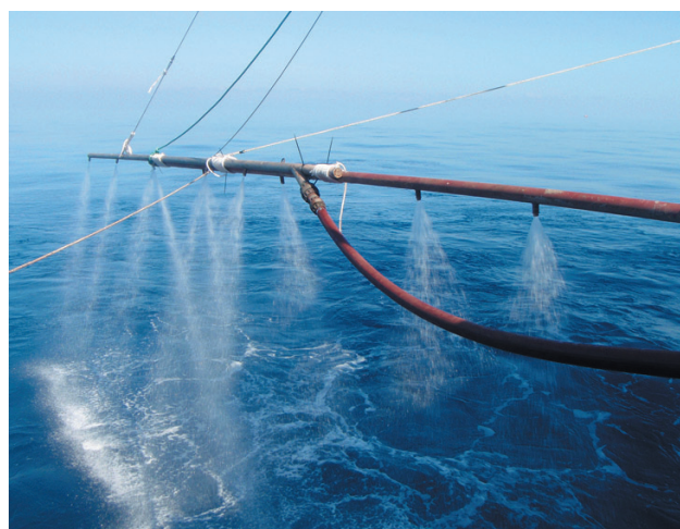
Dispersant spraying from a vessel-mounted spraying arm.
