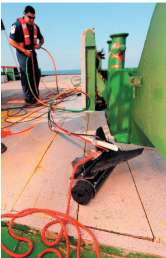
Preparation of a fluorometer to monitor dispersant effectiveness.
