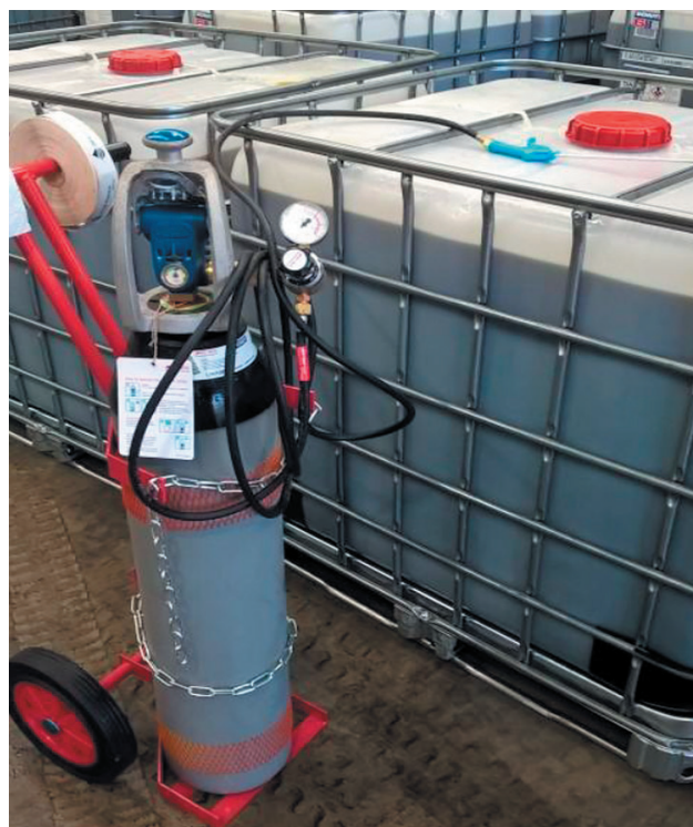
Equipment used to add nitrogen to an IBC and eliminate oxygen from the headspace above the liquid dispersant.
