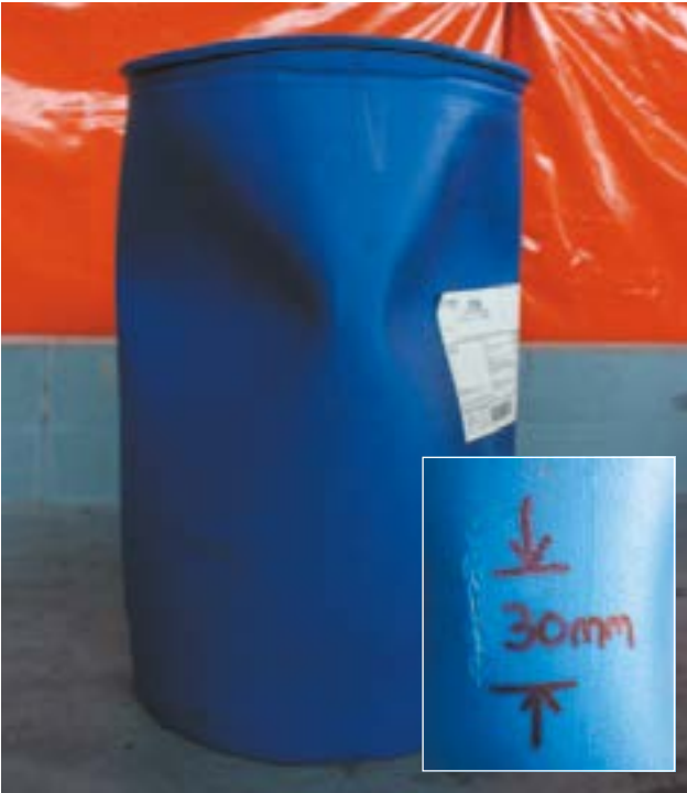
Splitting necks were observed on 25% of this stockpile of plastic drums after 10–20 years in storage. The specific cause was not known, but such damage could have an adverse impact on the product as it is likely to become exposed to the air.
