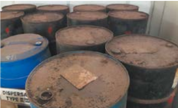
Steel drums showing signs of deterioration after 25 years. They were stored inside but occasional roof leaks caused water to pool on them which encouraged corrosion.
