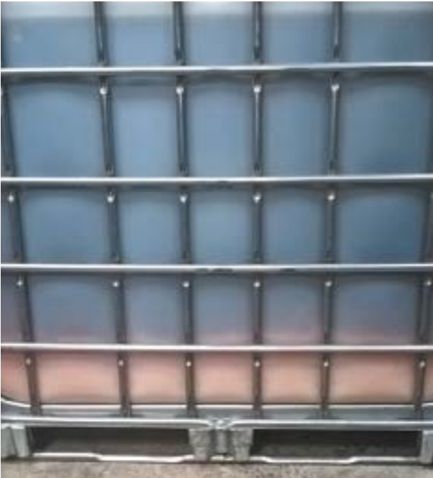
Above: an example of IBC deformation caused by loss of solvent; the product remained effective, but this can be prevented by the use of EVOH-HDPE laminated technology. Right: an example of visible residue formed during storage; in this case the residue remixed on pumping and did not affect the spraying equipment or product effectiveness.
